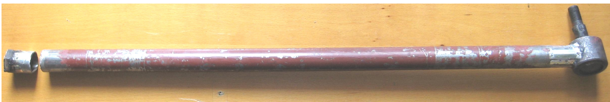
Fig. 8. Connecting rod with fatigue gauges after failure
