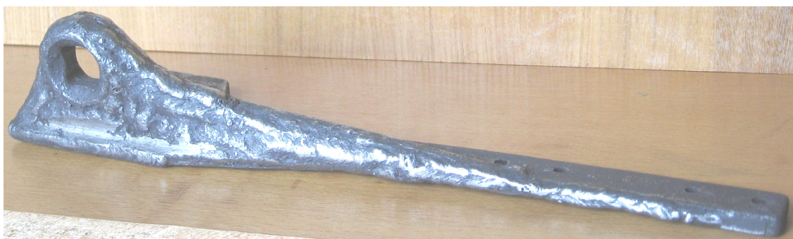
Fig. 2. Knife head after welding deposition
